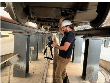
X750 Articulated Insertion Probes are **tungsten braided**, **resistant to heat up to 100°C and are corrosion resistant**. Tungsten braided probes are also scratch & abrasion resistant and waterproof up to 1-meter depth for 30 minutes with an IP67 environmental rating.
